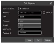
⑤ Click ■ to edit an IP camera as shown on the above left. Enter the new IP address, subnet mask, gateway, username and password of the camera. Click "OK" to save the settings.
